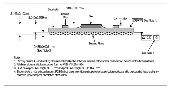
*Note:* Primary datum -C- and seating plane are defined by the spherical crowns of the solder balls.
